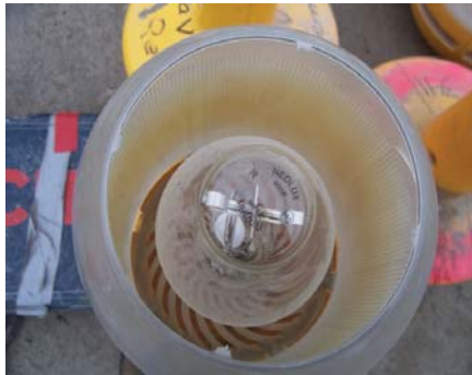
Wrong Bulb !!! Causes Fires !!!
